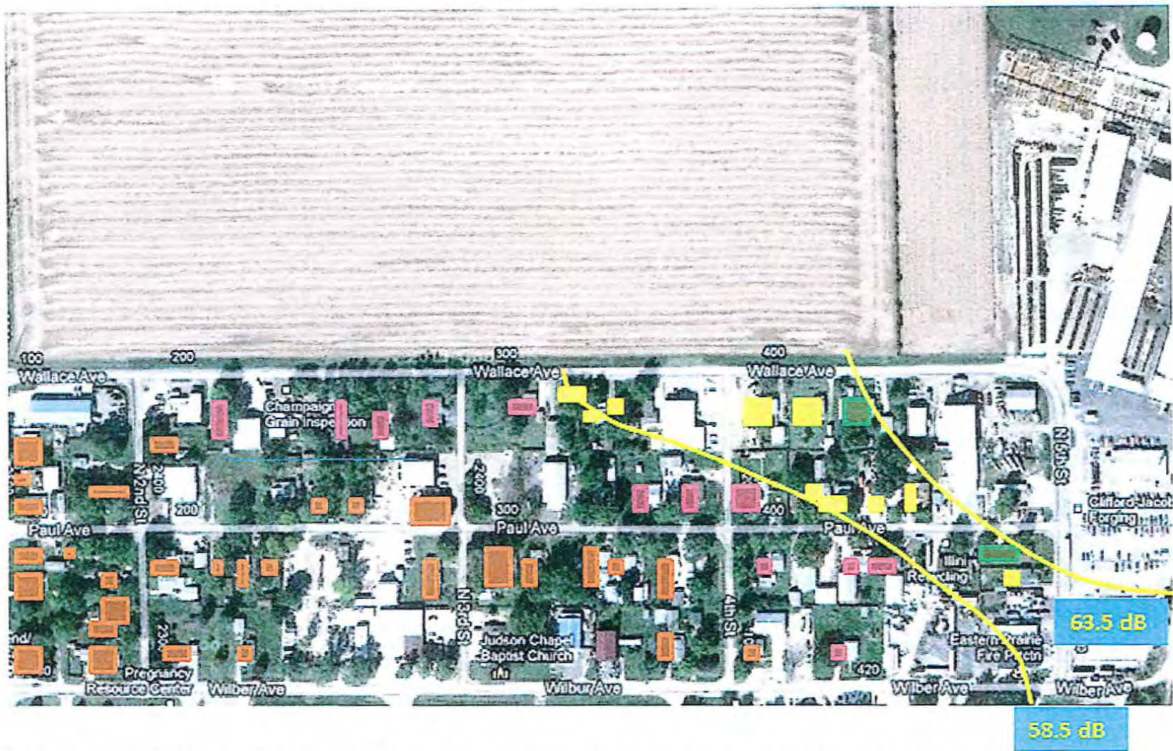
Figure E. A noise contour map showing the current 58.5 dB (A-weighted Leq) contour with affected residences marked; there are twelve houses used as residences that are in excess of 58.5 dB, and two of these are at or in excess of 63.5 dB (A-weighted Leq).
