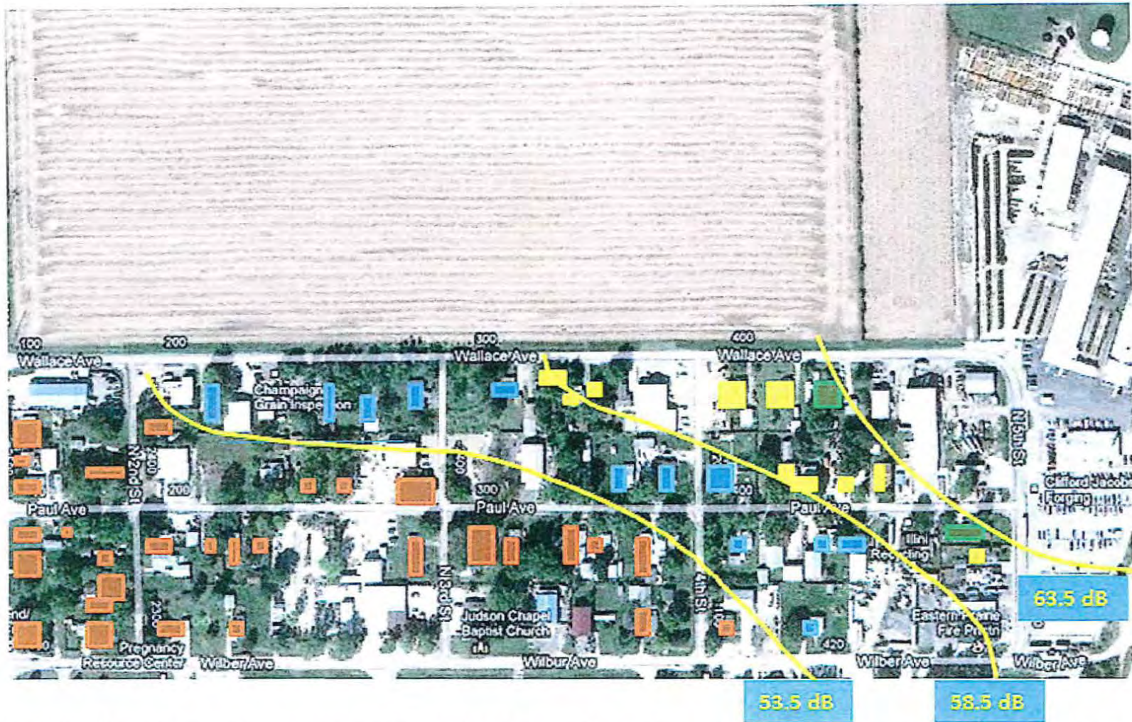
Figure F. If Petitioner's proposed operational levels go forth, 24 houses (blue, yellow, and green) used as residences will be at or in excess of the 53.5 dB (A-weighted Leq) nighttime limit, and of these, 12 (yellow and green) will be at or in excess of 58.5 dB (A-weighted Leq) daytime limit, and of those twelve, two (green) will be at or in excess of 63.5 dB (A-weighted Leq).
